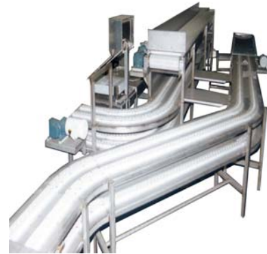
Pan Conveyor System
